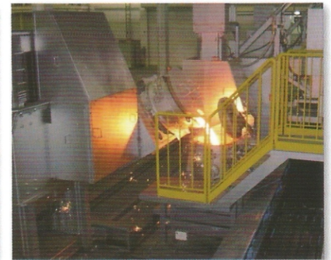
Molten metal transfer from transfer carriage to pouring ladle. (Left: Transfer carriage, Right: Scene from pouring ladle)
