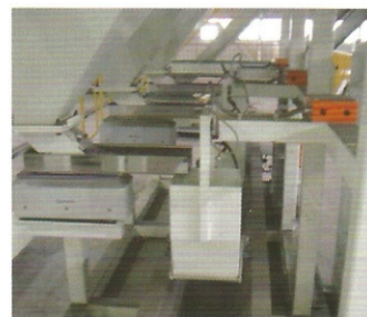
Accurate inoculant feeding by electromagnetic feeder and load cell.
